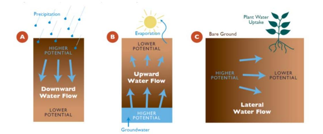
**Figure 2-1: Three basic pathways of water movement through the soil profile (Source: McCauley 2005).**
