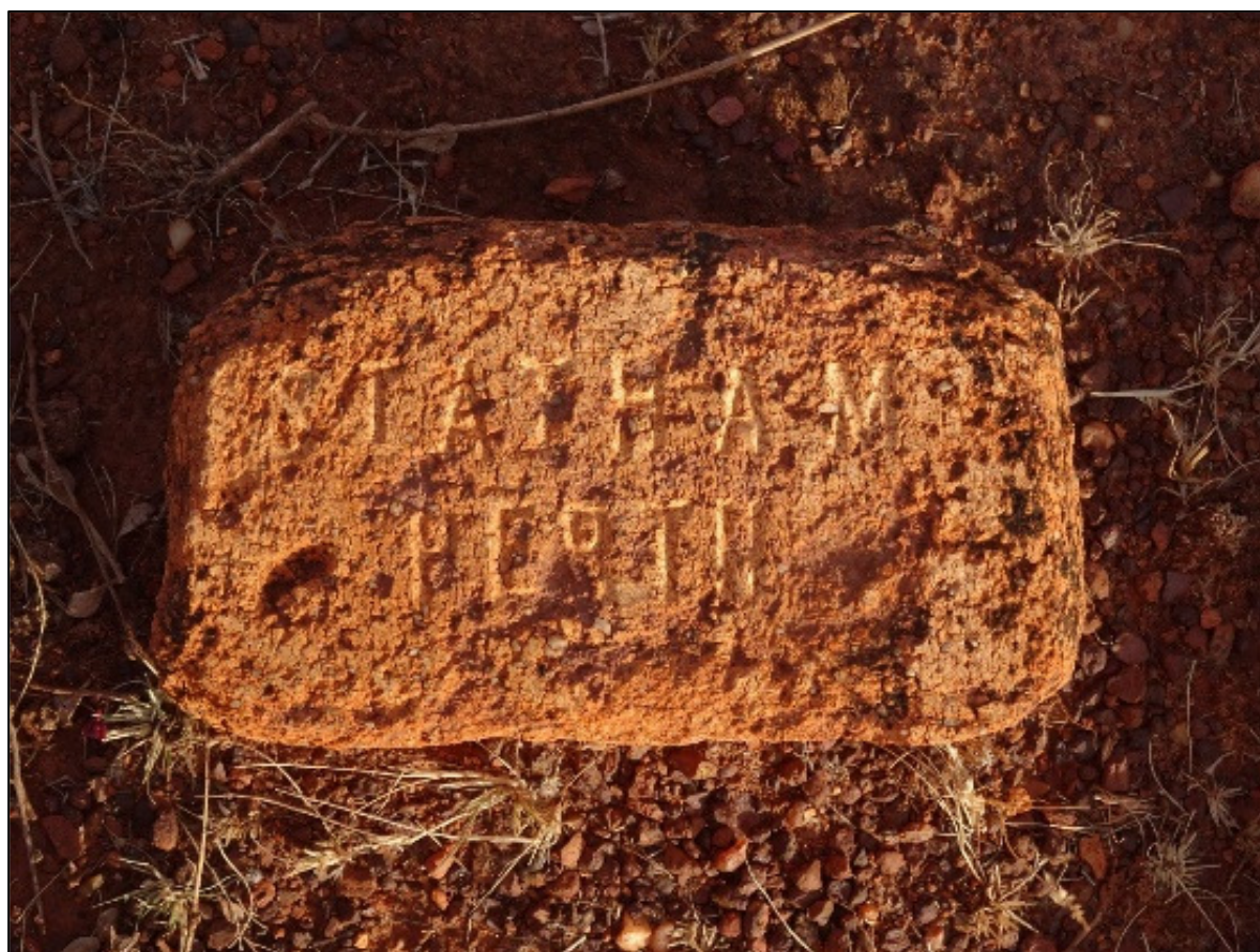
Figure 30: A machine-made brick stamped Statham Perth. ID234
