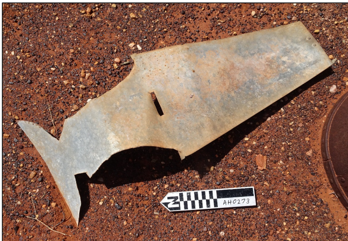
Figure 56: A sheet of flat galvanized iron that was used for a primary purpose and was later recut to make a windmill vane. ID778.
