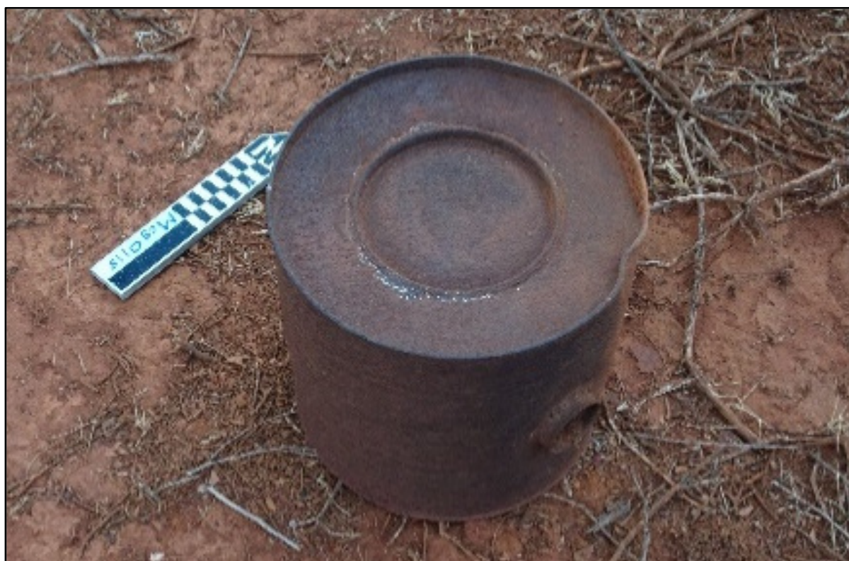
Figure 31: An ferro-based container with a welded inlet/outlet. ID239.
