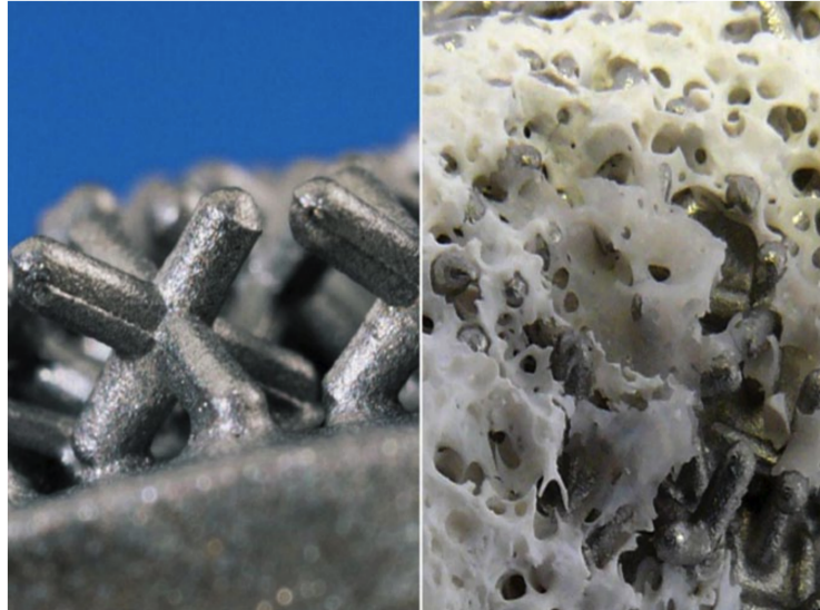
Figure 26. Magnified image of the Spongiosa Metal® surface showing that this structure is part of the implant core rather than being a coating. Osseointegration showing the bony penetration.
