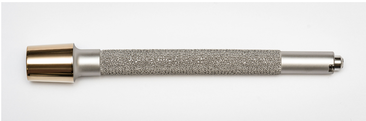
Figure 29. Newly designed ILP implant. Reintroduced based on my design inputs featuring a completely smooth distal transcutaneous region that is highly polished and coated with a TiNbN ceramic layer to achieve minimal friction to the skin.
