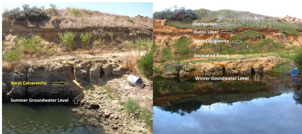
Figure 3-10: Cross-section of the soil and karst calcarenite layer from one of the irrigation ponds.
