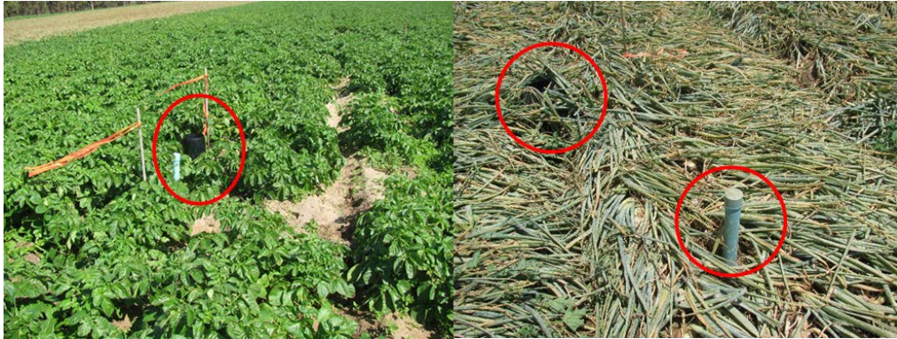
Figure 5-5: The rain gauges situated under foliage within a potato crop (left) and in an onion crop (right).
