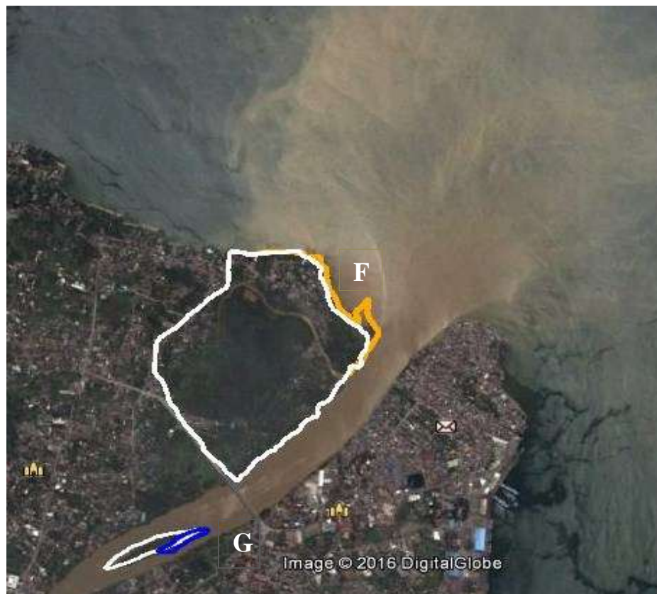
Figure 4.9: Temporal changes (2004–2015) along Cagayan River and its mouth showing land progression (F - yellow) and land erosion (G - blue) due to river sedimentation and human intervention (base map from Google Earth, 2015).
