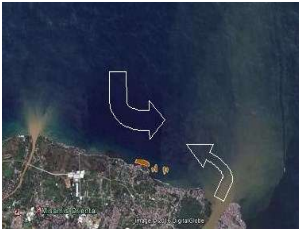
Figure 4.21: CdeO River plume westward expansion, threatening the Bonbon coral reefs and east-bound currents potentially transporting sediment from Iponan River (far west) towards the reef site (base map from Google Earth, 2015).
