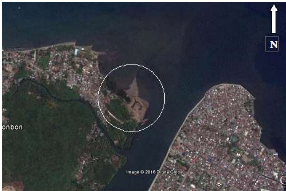
Figure 3.39: The map shows a land mass (inside the circle) at the right corner of the river mouth that came from from sediment materials dredged from the river mouth bottom. The prograded land mass is planted with mangroves and some parts remain bare due to the dumping of dredged materials. Other accreted land along the coast and banks was compacted with dredged materials for housing purposes (base map from Google Earth, 2015).
