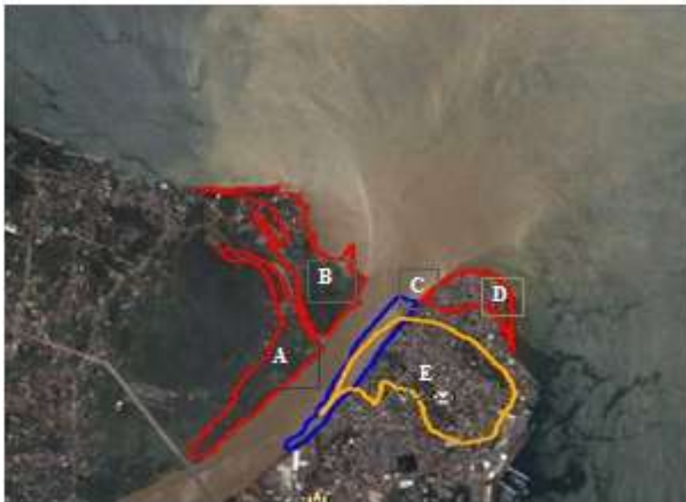
Figure 4.8: Physical and biological changes (1932–2015) within the Cagayan de Oro River mouth and vicinity showing land progression (red); land regression (blue) and land conversion (yellow) due to natural processes and human intervention (sources: 1957 NAMRIA map and Google Earth 2015 base map).
